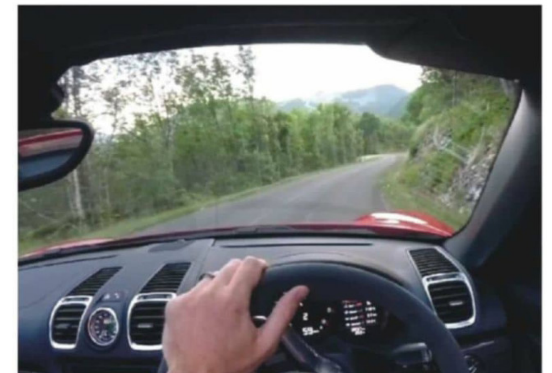
Corner Exit Squeeze the throttle progressively as you smoothly unwind the steering in an effort to gain rear grip
