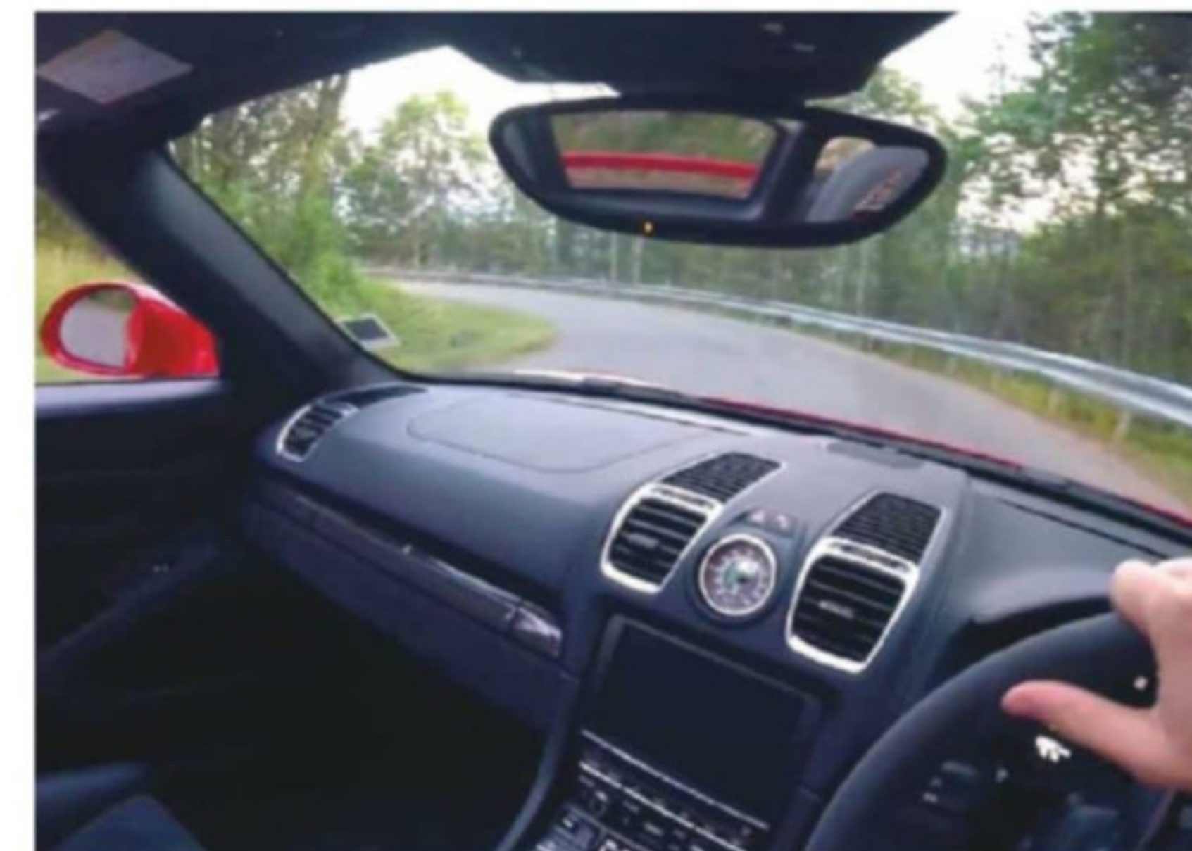
Corner development Steer slowly and progressively in order to transfer load to the outside front tyre
